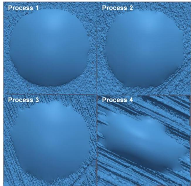
Fig. 7: Numerical analysis of shape of the droplets deposited on ceramic surfaces, top view of lattice Boltzmann simulation (drop volume  $4 \mu\text{l}$ , density ratio 36, static contact angle  $\theta=45^\circ$ , Shan-Chen model intermolecular interaction parameter  $G=-6$ ).
