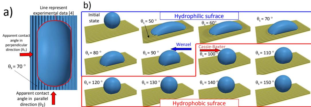
Fig. 1. (a) Validation of lattice Boltzmann method, where red contour corresponds to experimental data ; (b) Anisotropic wetting ( $\theta_s = 50 - 90^\circ$ ) in Wenzel state for hydrophilic surfaces and quasi-isotropic wetting ( $\theta_s = 100 - 150^\circ$ ) in Cassie-Baxter state.
