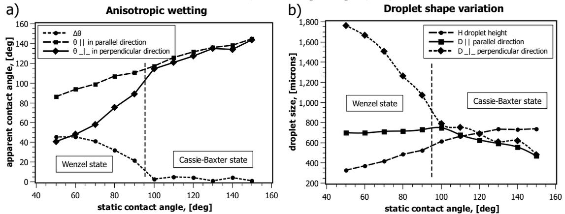
Fig. 2. (a) Influence of  $\theta_s$  of textured surface on anisotropic wetting:  $\theta_{||}$ ,  $\theta_{\perp}$ ,  $\Delta\theta = \theta_{||} - \theta_{\perp}$ , where  $\theta = 2 \arctan(2H/D)$ ; (b) Droplet shape variations as a function of  $\theta_s$ :  $H$ -droplet height,  $D_{||}$ -solid-liquid contact size in parallel direction,  $D_{\perp}$ -solid-liquid contact size in perpendicular direction.
