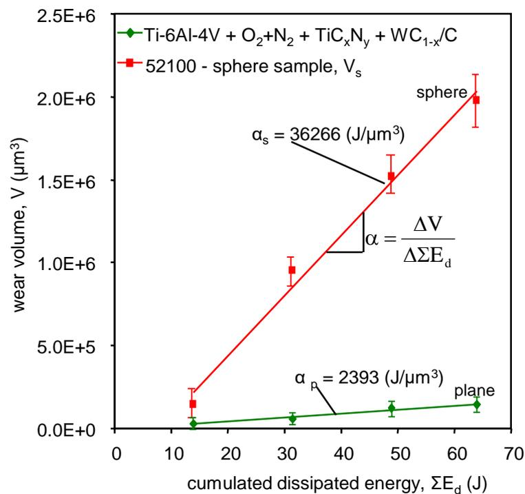
Fig. 8: Linear evolution of wear volume ( $V$ ) as a function of cumulated energy dissipated in contact during the test  $\Sigma E_d$ , for the multilayer system on Ti-6Al-4V alloy with external nanocomposite carbon-based  $\text{WC}_{1-x}/\text{C}$  layer against 52100 sphere.
