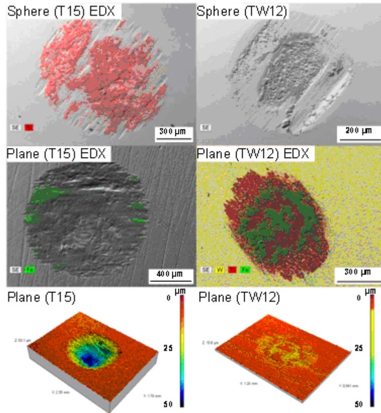
Fig. 10: Wear scar: SEM images and 3D morphologies of uncoated Ti-6Al-4V // 52100 tribosystem and multilayer system on Ti-6Al-4V alloy with an external nanocomposite carbon-based WC<sub>1-x</sub>/C layer against 52100 sphere (displacement amplitude  $\delta^*=100 \mu\text{m}$ ).
