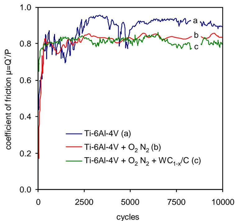
Fig. 5: Analysis of friction evolution for untreated (Ti-6Al-4V), hardened (Ti-6Al-4V + O<sub>2</sub> N<sub>2</sub>) and coated (Ti-6Al-4V + O<sub>2</sub> N<sub>2</sub> + WC<sub>1-x</sub>/C) in sphere/plane contact configuration, displacement amplitude  $\delta^* = 50 \mu\text{m}$ .
