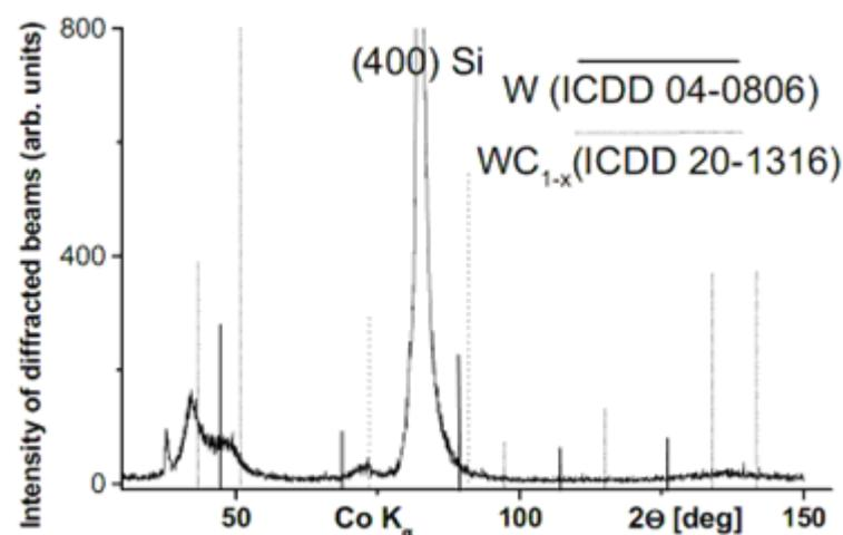
Fig. 4: Results of X-ray phase analysis of WC<sub>1-x</sub>/C coating deposited on the silicone substrate, nanocrystallites of WC<sub>1-x</sub> phase in an amorphous carbonaceous a-C matrix [23].
