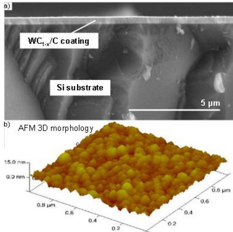
Fig. 3: Characterization of the new WC<sub>1-x</sub>/C coating deposited by reactive magnetron sputtering on the silicone substrate, a) SEM image of coating fracture and b) AFM morphology of coating surface [23].
